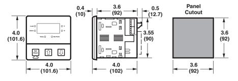
Figure 3.3 Mounting Dimensions
